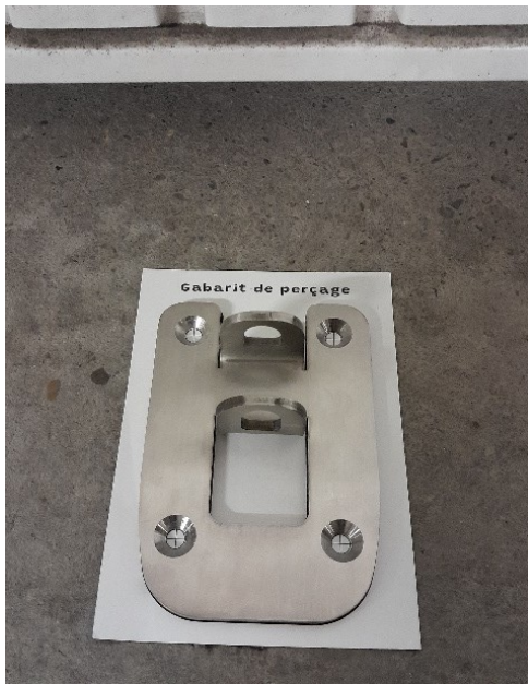
Configuration 1 : the 2 loops of the plate face the door side
