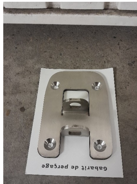
Configuration 2 : the template is rotated half a turn compared to configuration 1
